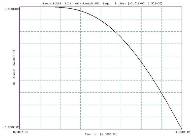
Figure 8: Probe plotting capabilities for the WALKTHROUGH example. Calculated magnetic field B_z(t) just outside the aluminum vacuum tube at z = -2.00 in.
