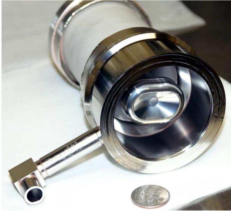
Figure 1: Electron gun assembly.
