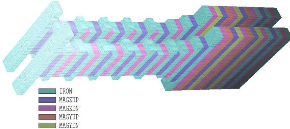
Figure 8: Periodic-permanent-magnet assembly.
